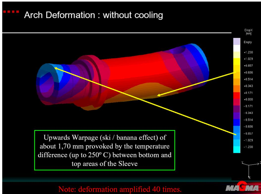
Figure 11. Result of simulation showing upwards arch deformation (in X axis with 40 x amplification) caused by high temperature difference between superior and inferior are of the shot sleeve.
