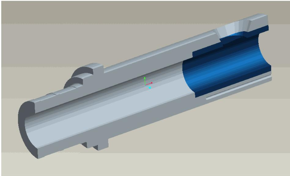
Figure 2. Image of modeling with cross section showing the tungsten sleeve (blue) in the pour hole area.
