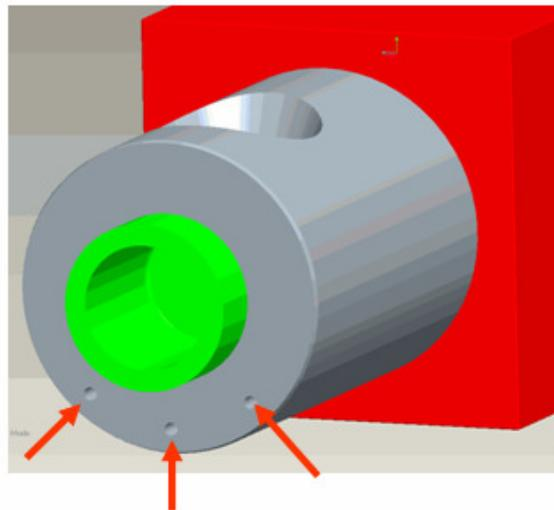
Figures 3 and 4. Cooling jacket at the biscuit area and cascade cooling lines in the pouring hole area.
