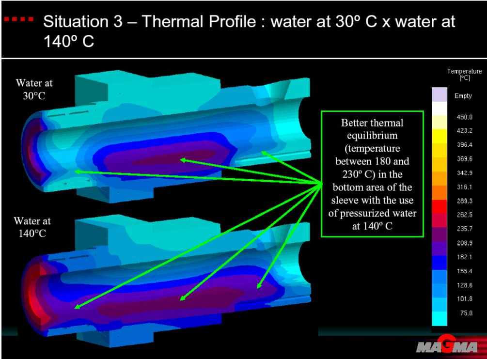
Figure 7. Results of simulation showing better thermal balance in the lower area of the shot sleeve, using water at 140° C in comparison with the anterior situation (water at 30° C).
