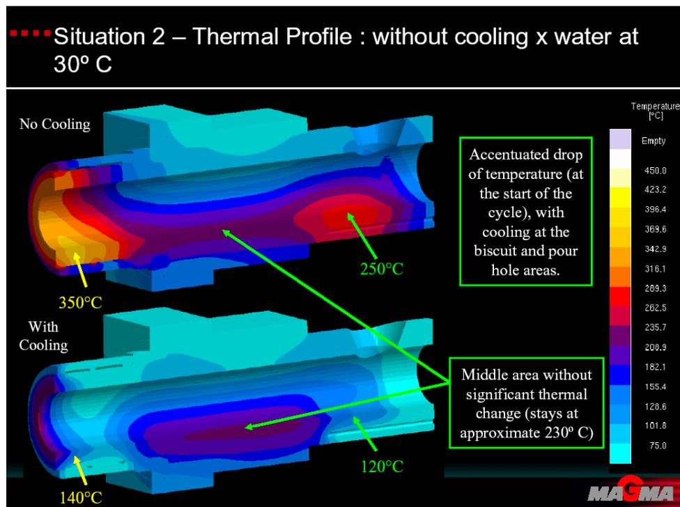
Figure 6. Results of simulation showing high degree of heat removal in the pour hole and in the biscuit area, with the application of cooling in comparison with anterior situation (without cooling).
