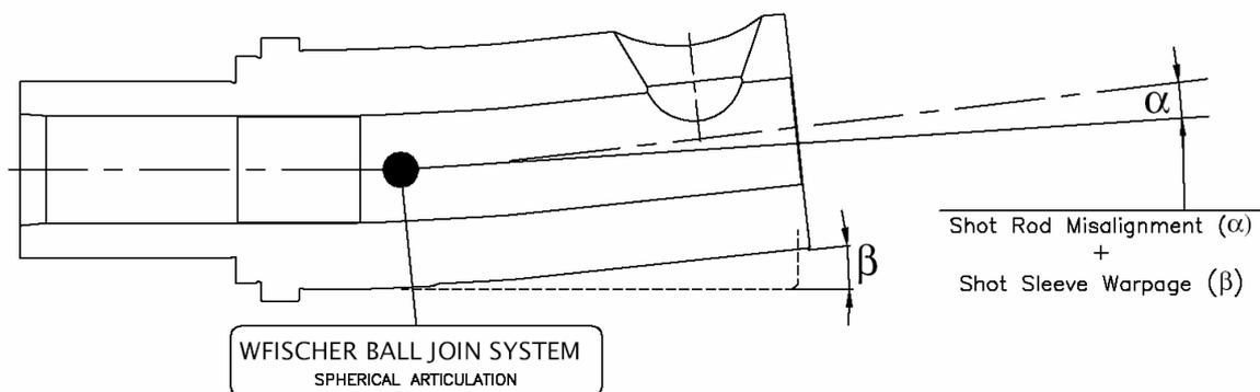
Figure 13. Demonstration of compensation of the upwards arch deformation and misalignment between shot rod and sleeve by the use of the plunger tip with articulating system.
