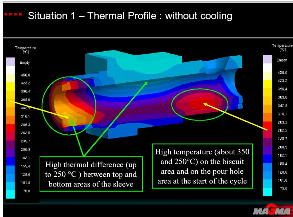
Figure 5. Simulation results showing high heat concentration in the pour hole and biscuit areas as well as high temperature difference between higher and lower areas, without use of cooling.
