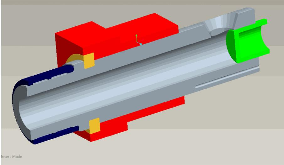
**Figure 1. Image of modeling with cross section showing the shot sleeve (grey), flange (yellow), plunger tip (green), cooling jacket (blue) and fixture component (red).**
