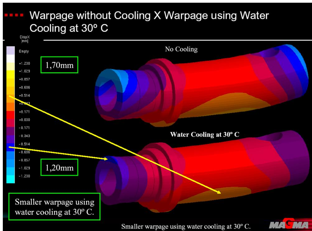
Figure 12. Result of simulation showing reduction on upwards arch (on X axis, 40 x amplification) with water cooling in the ends of the shot sleeve in comparison with anterior situation (without water).
