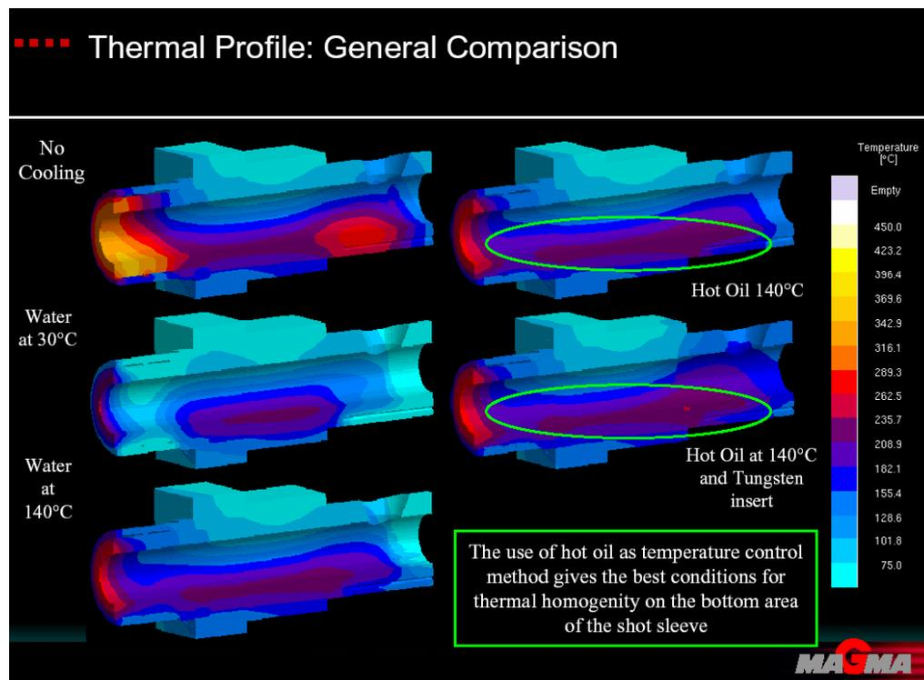
Figure 10. Comparison of all 5 situations of simulation, showing the advantage of the use of the hot oil for the thermal balance of the lower area of the shot sleeve.
