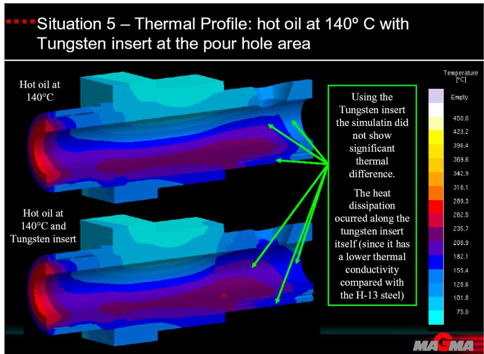
Figure 9. Results of simulation showing no significant thermal difference in the lower area of the shot sleeve, with oil at 140° C and tungsten sleeve in comparison with anterior situation (oil at 140° C without tungsten sleeve).
